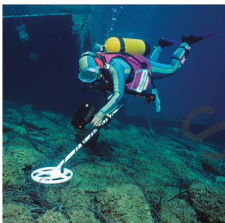
FIGURE 7.2.2 A diver using a metal detector. If a metal object is found underneath the coil of the detector, an emf will be induced which creates a current that will affect the original current. The direction of the induced current is predicted by using Lenz's law.
