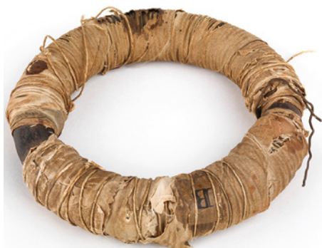
FIGURE 7.1.1 Michael Faraday's original induction coil. Passing a current through one coil induces a voltage in the second coil by a process called mutual inductance. This coil is now on display at the Royal Institution in London.
