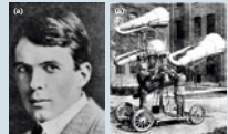
Figure 2.2.4 (a) William Lawrence Bragg, winner of the Nobel Prize for Physics 1915 and developer of sound ranging methods. (b) An acoustic locator. The large horns amplified distant sounds, monitored through headphones worn by a crew member.
